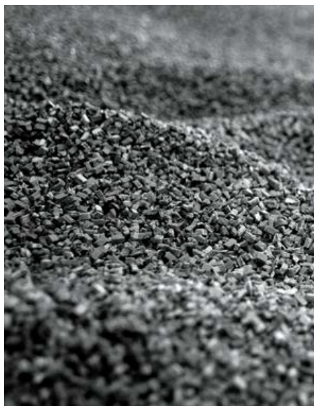
Recycled underlay is manufactured using recycled rubber crumb, sourced from worn tyres
