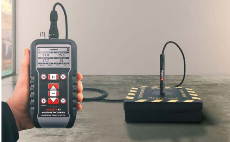
A British Standard Hood test in use with plug-in hygrometer probe
