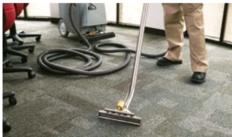
BOTTOM: Wet slurry extraction using a wet vacuum. This is an effective way of removing wet cleaning slurry from all types of floor surfaces and is especially useful in smaller areas following manual mopping and rinsing.
