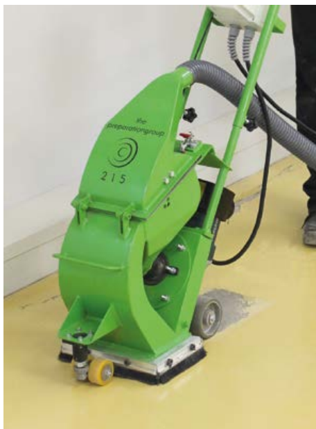
ABOVE: Shotblasting is the most economical method for removing glaze/laitance from power floated concrete, texturing and cleaning concrete or tiled surfaces and for removing paints and sealants
